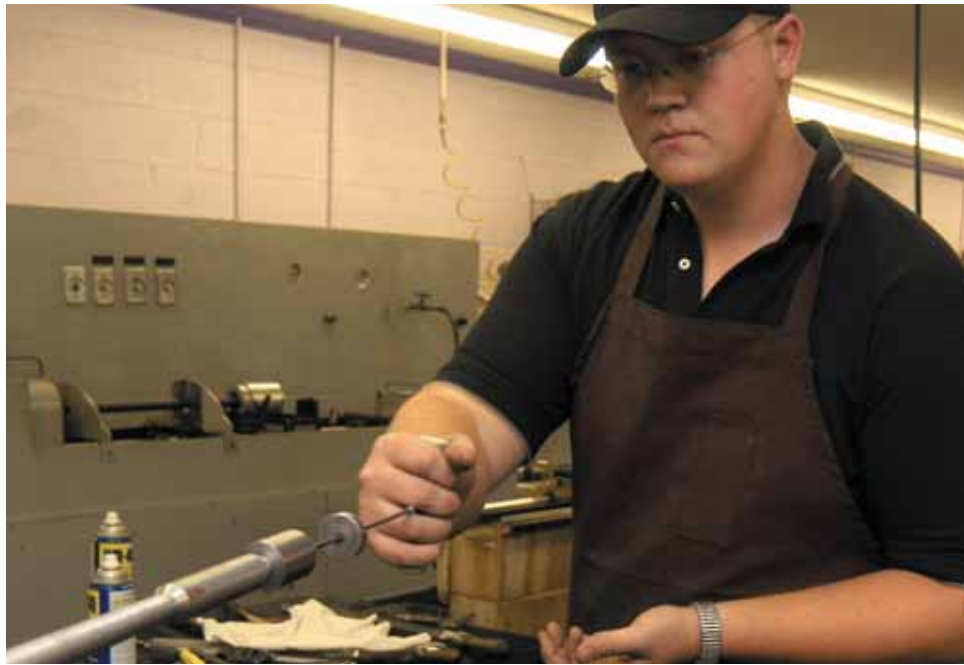
Cain Jarrett "laps" a barrel to polish away minute imperfections. (Photo courtesy of Jarrett Rifles)
